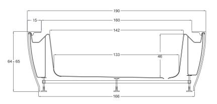
If the bath is recessed the masonry cannot reenter more than 1 cm with respect to the external edge of the bath. An inspection panel and air intake must be installed.
